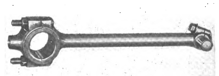
Fig. 5—Tubular form of connecting-rod, showing extension at lower end for balancing
